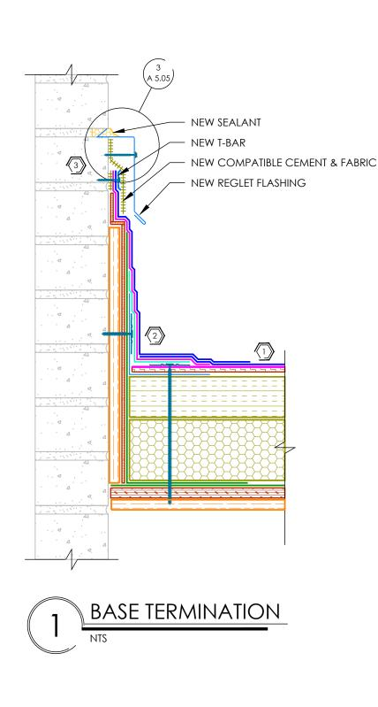
REMOVE MORTAR FROM JOINT TO A DEPTH OF 5/8" [16mm] MIN
